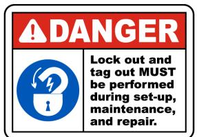
For good safety a lock out tag must be performed during set -up, maintenance and repair of the machines. This eliminates the possibility of someone else to connect the electrical service and starting the machine while under maintenance.
