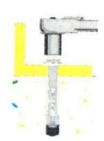
Select a carbide drill bit with a diameter equal to the anchor diameter. Drill hole to any depth exceeding the desired embedment.
