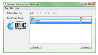
• In the example above, you can see that FM7 equipped machines will show up listed by model and serial number (ex. "HE60-002222" in the picture above). Other com ports, like an adapter used to program the EL6, will show up identified by the com port number (ex. "COM3" in the picture above). To find the model and serial number of any B&C washer-
