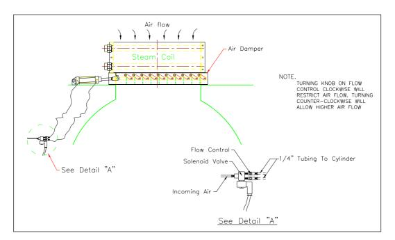
Figure.3-7 Steam Damper Air Cylinder Adjustment
