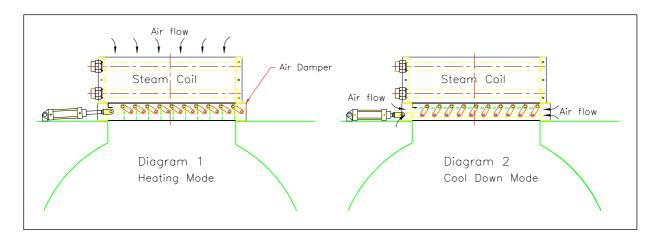
Figure.3-6 Steam Damper System Operation
