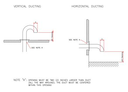
Figure.3-2 Outside Duct Work Connection
