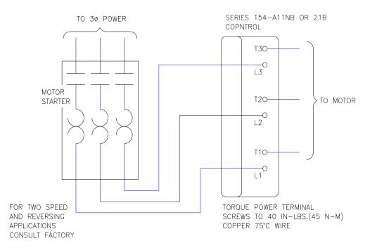
When the motor starter is turned on, 3-phase  $(3\emptyset)$  power will be applied to the input to the controller. The controller will then ramp up the voltage to the motor. The duration of the ramp will
