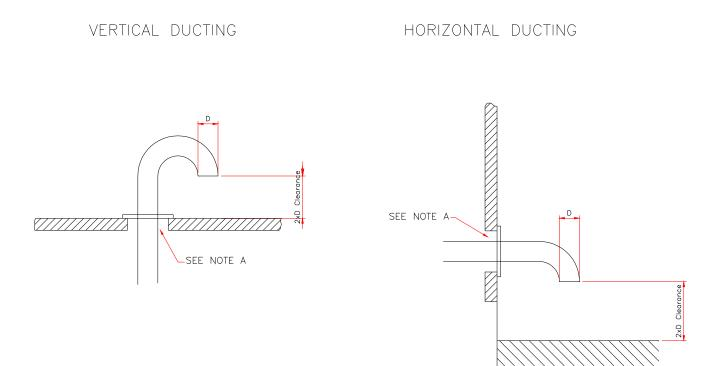
NOTE "A": OPENING MUST BE TWO (2) INCHES LARGER THAN DUCT (ALL THE WAY AROUND). THE DUCT MUST BE CENTERED WITHIN THIS OPENING
