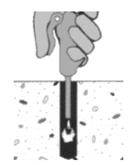
Clean hole or continue drilling to accommodate drill fines (concrete dust). Please wear eye protection.
