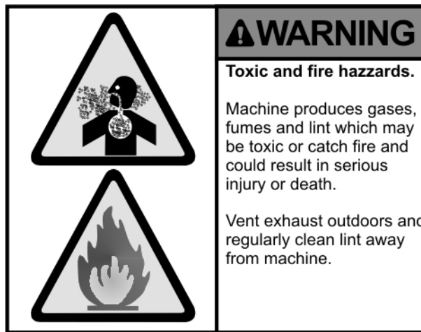
Figure 3.4: IS Series - Proper Exhaust is critical for safety!
